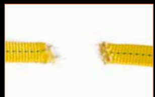
SHARP EDGE FAILURE: Traditional webbing lifeline
