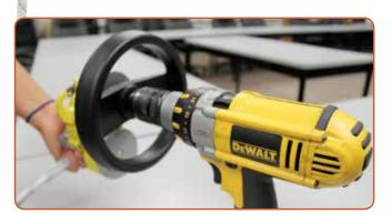
Protrudring 10 mm diameter shaft on the hub is used as a drill adaptor. Connect the Power Drill to help control the pace and / or raise the fall victim. Min advised torque: 45 N.m. Min rotating speed: 0-300 turns/min
