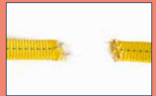
SHARP EDGE FAILURE: Traditional webbing lifeline
