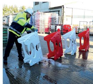
To empty, lift the end of the barrier furthest from the filling aperture and rest on the ground until the water ceases to flow.
