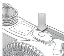
By briefly pressing the button it is possible to switch between two air flow levels: 160 L/min and 210 L/min. The maximum air flow mode provides a higher protection level for the user. However, a higher flow rate may be unpleasant at low temperatures.
